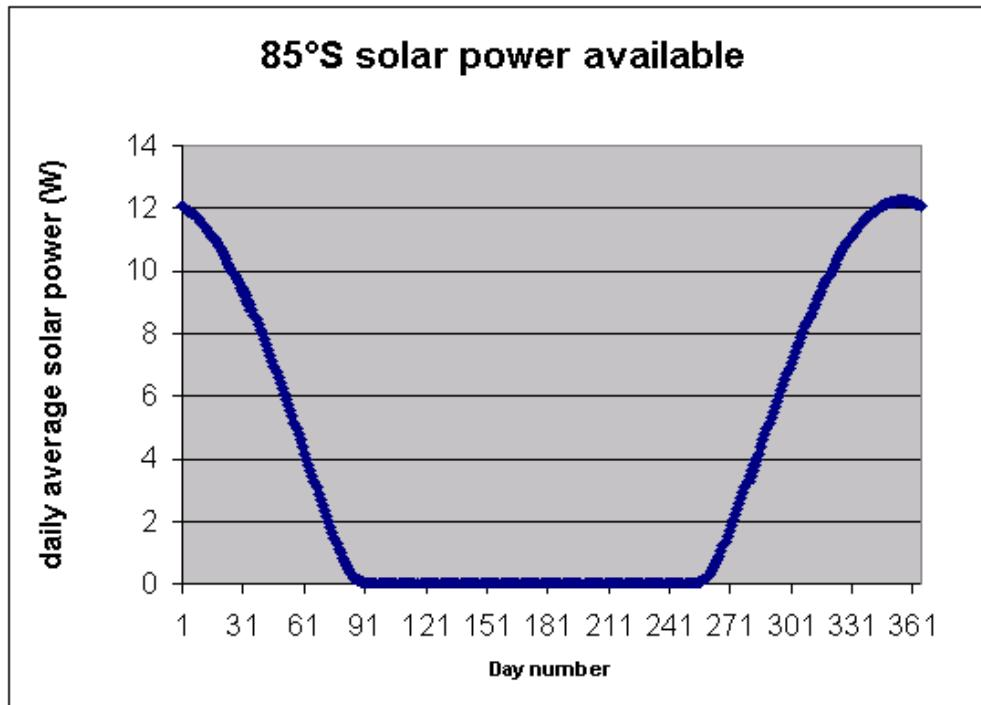
With two battery boxes (total capacity 400Ahr), this amount of solar power and a 0.5W average power usage results in less than 50% of the battery capacity being used in the depth of winter.
